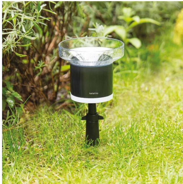
Figure 2: Netatmo rain gauge with tipping bucket mechanism, part of the popular Netatmo PWS. Setup, placement and update interval depends per rain gauge [Netatmo, 2020b].
