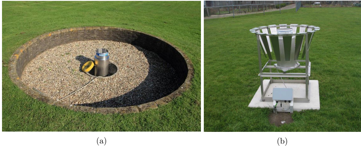
Figure 1: Different rain gauge setups to minimize wind influence [Brandsma, 2014]. (a) KNMI pit gauge setup. (b) Wind screen setup used at some KNMI stations and by several water boards.
