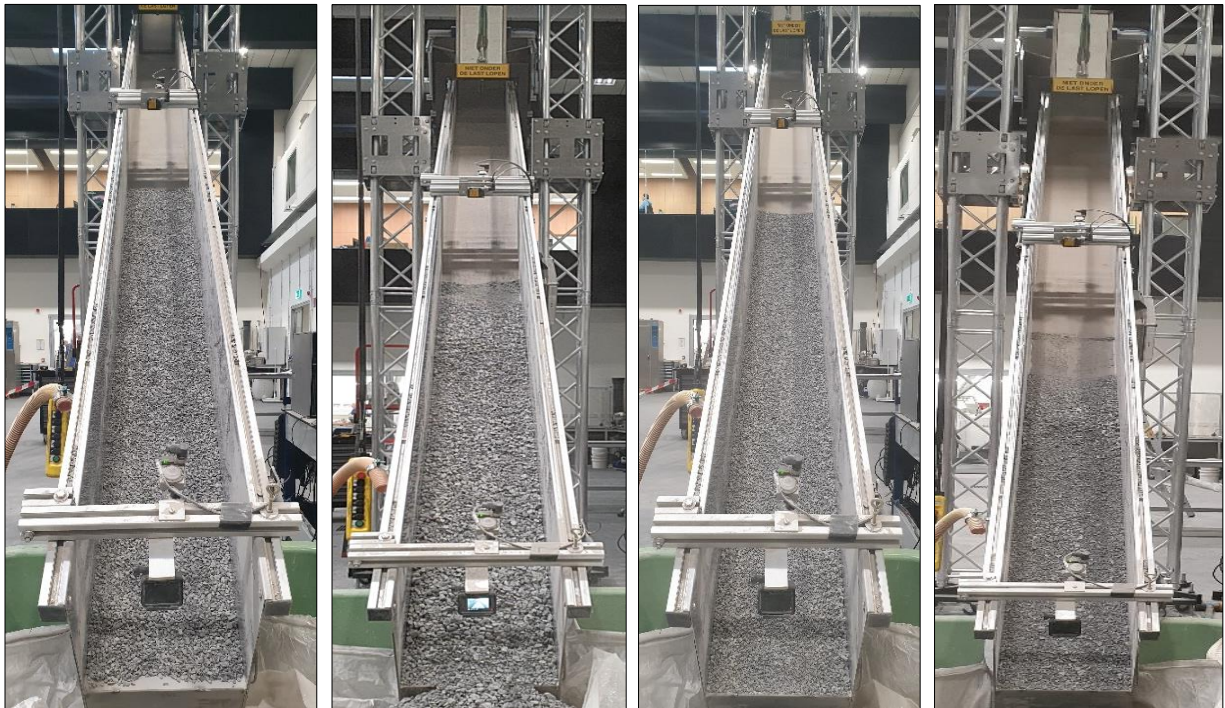
Figure 4.9 The erosion in a different flow composition: (a) Before experiments; (b) Coarse-grained flow (Test68); (c) Fine-grained flow (Test54); (d) Mixed flow (Test99).
