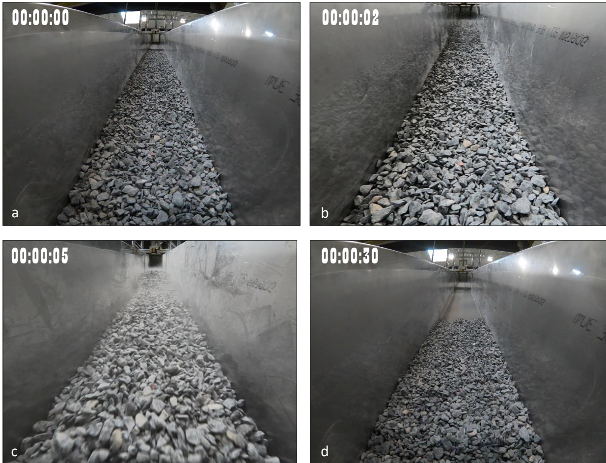
Figure 4.7 The erosional mechanism: (a) Before experiment; (b) The initiation phase; (c) The motion phase; (d) The deposition phase; The flow travel time is 30 seconds for each experiment.
