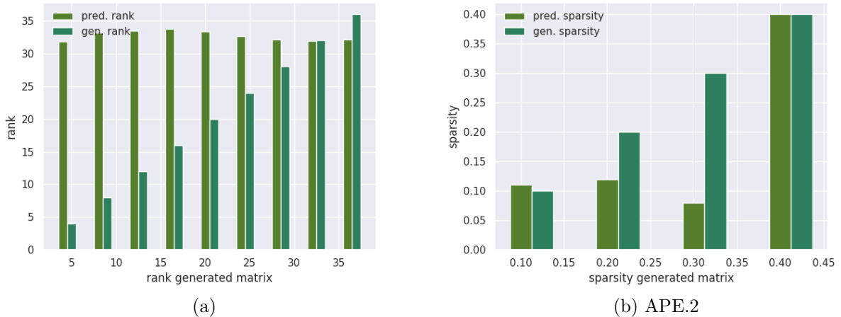
Figure 3: Average best performance of SGD for matrices generated of different ranks (left) and sparsities (right).
