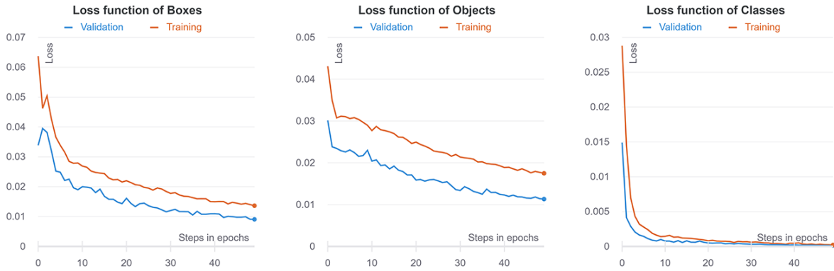
Figure 17: Panels showing the progress of the training phase. The Box, Object and Class graphs show the loss functions which should be as low as possible.
