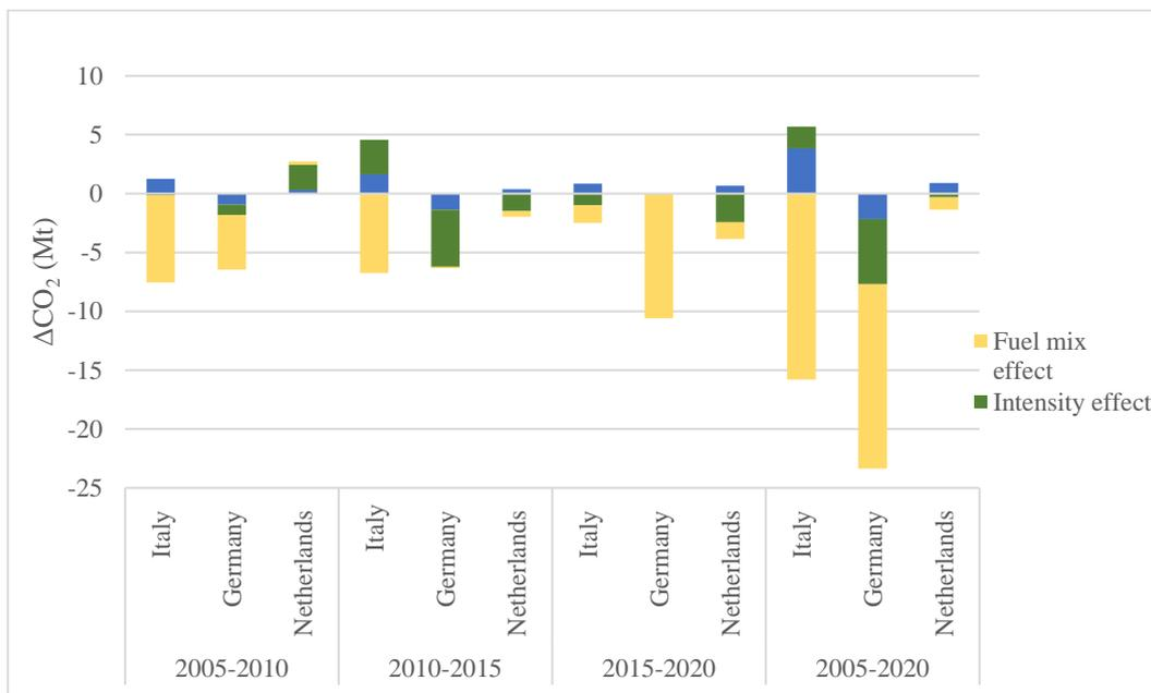
Figure 14, Decomposition analysis results for the analysed MS emissions in the Residential and buildings sector between the period 2005-2020 (Source: PRIMES 2016).
