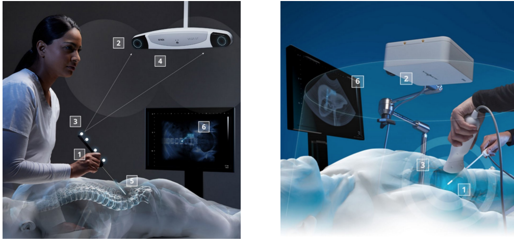
(a) Example of optical tracking system for freehand US. (b) Example of EM tracking system for freehand US.
