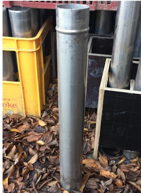
Fig. 6. The thin-walled sample tube of 0.5m length used for retrieving undisturbed soil samples.
