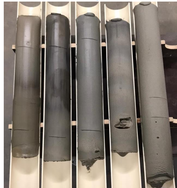
Fig. 8. Undisturbed soil samples taken at B03. The samples were pushed out of the sample tube onto half-open PVC pipes.
