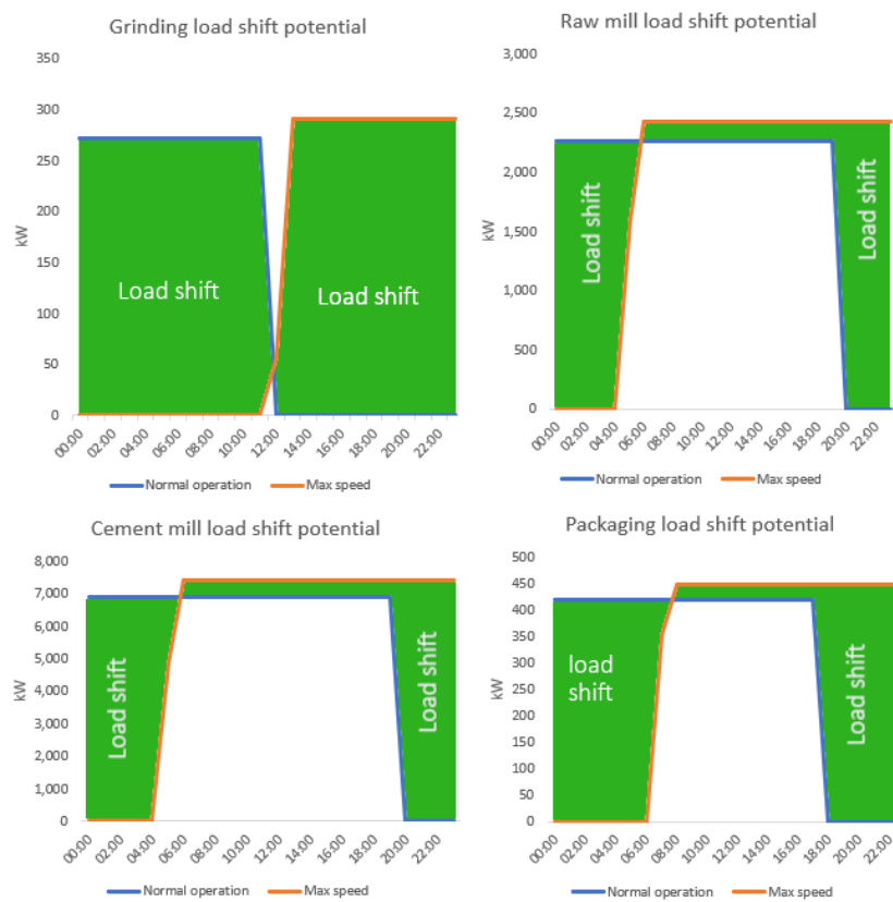
Figure 30: Daily load shift potential generic cement production processes. It should be noted that due to the software used to plot the graphs the lines appear to be skewed while they should be vertical.
