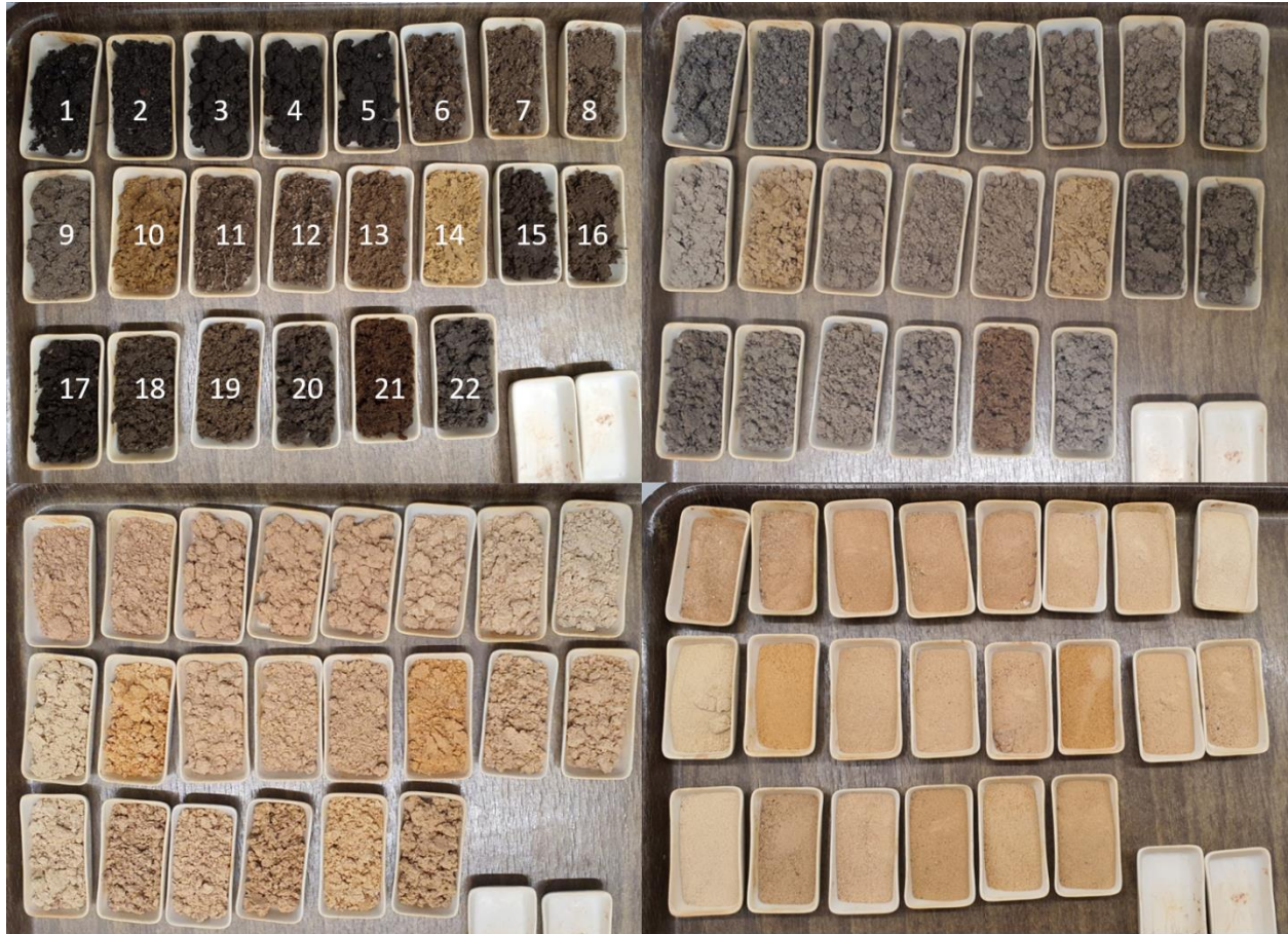
Figure 16. Top left: Samples 1-22 shown as they looked after post-fieldwork refrigeration. Top right: Samples after they were dried overnight. Bottom left: Samples after being heated in the furnace for LOI analysis. Bottom right: Dried samples after LOI analysis and after being ground to break aggregates.
