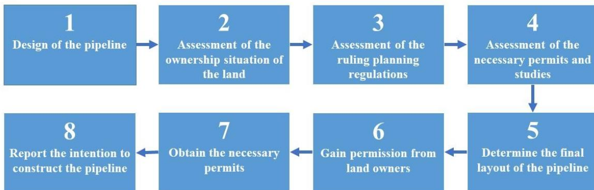
Figure 5: Eight steps of planning a pipeline. Source: own work, based on Lindenbergh, et al. (2018).
