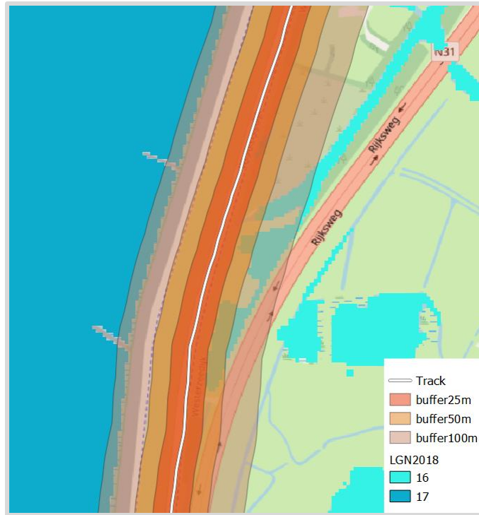
Figure 3.9: Surface water represented 5 \times 5 pixels intersecting with 25, 50 and 100m buffers of a GPS track. In LGN, class 16 corresponds to salt water and 17 demonstrates fresh water.
