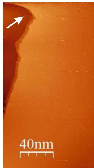
Figure 8: An AFM image showing the bending (marked by the arrow) of a step height of a Si surface caused by piezo creep. Adapted from Voigtländer.<sup>18</sup>
