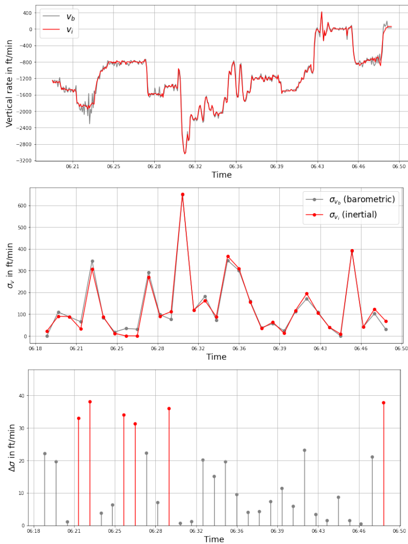
Figure 3.2: Descending aircraft. Top: two sources of vertical rate. Middle: standard deviations of v_b and v_i in time segments of one minute. Bottom: absolute difference in standard deviation with detected turbulence in red.
