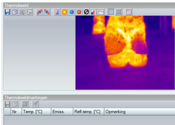
Figure 4: IRT image from Testo IR Soft 4.3 software. The program provides no information over the image as a whole.
