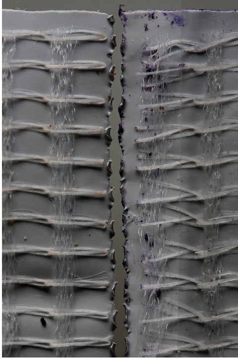
Figure 2.7.: Photo of the yarns of part of the edges of two pieces of torn duct tape under a microscope. The horizontal yarns are warp yarns and the vertical yarns are the weft yarns. [25]
