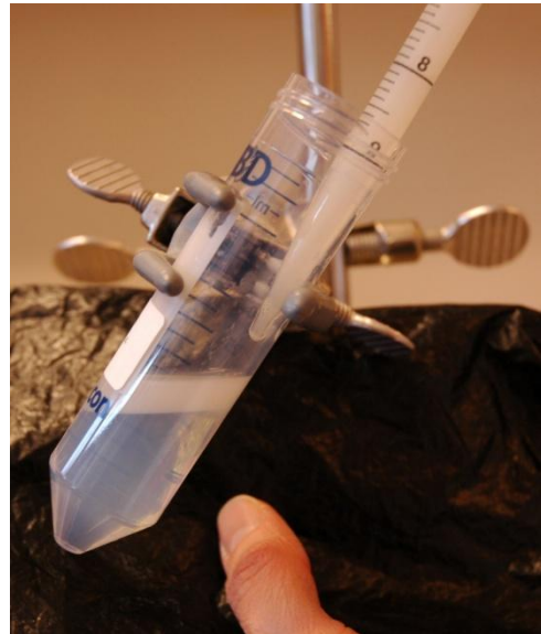
Picture 2: preparation of tubes; Colloid layer on the bottom of the tube and semen aliquot is pipetted on top of it.
