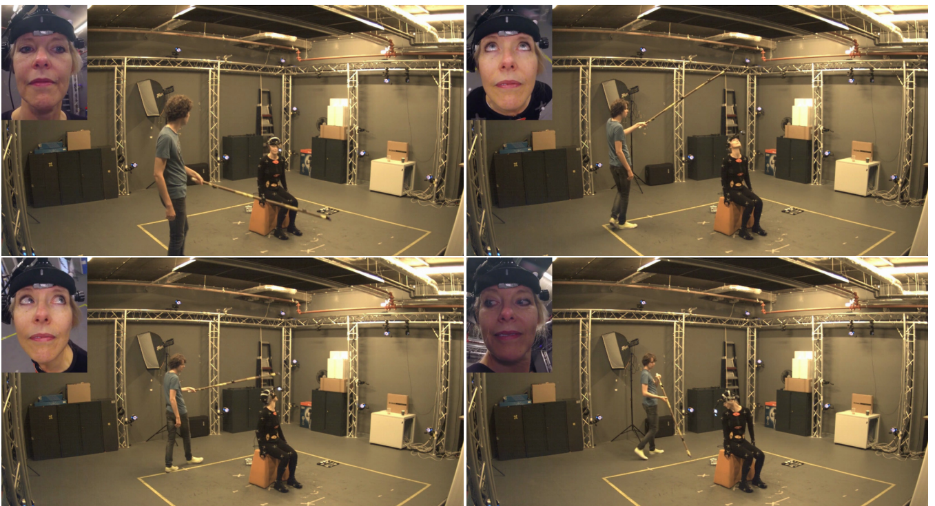
Figure 11: Images of the motion capture recording in a sitting pose, with the head-mounted camera footage in the top-right corner.
