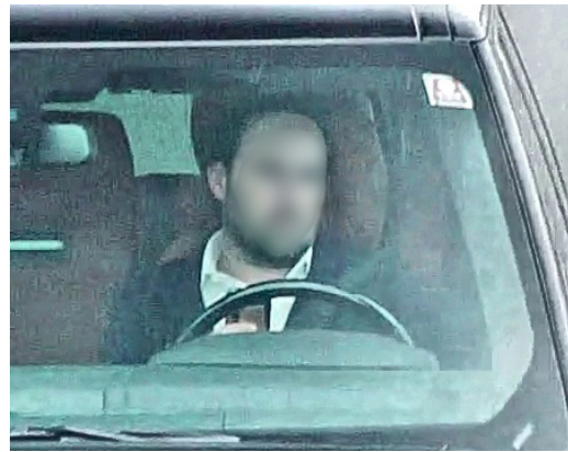
(b) The second type of false negative. The phone is clearly visible, but the hand holding it is only very slightly visible. If no hand is detected in this image, the phone will be classified as being in a phone mount due to its distance from hands or faces.
