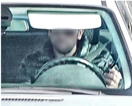
(a) The first type of false negative. The phone is a small part of the image, due to its orientation. It is also partly occluded and the hand holding the phone is positioned and oriented slightly nonstandard.
