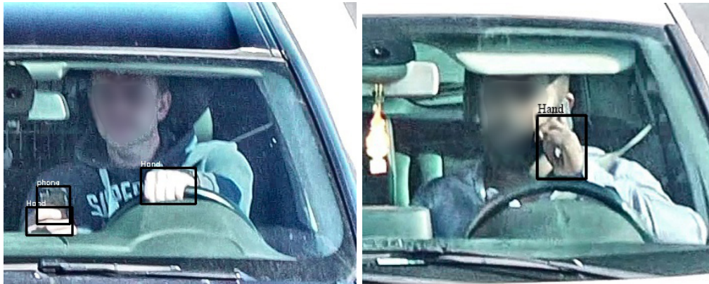
Figure 7: On the left a situation in which the phone and hand detector works well. Everything is correctly detected. On the right only a hand is detected, but the partly occluded phone is not.
