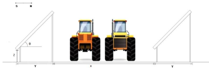
Figure 1: Agrivoltaic system in which the PV-panels are mounted on the ground. The space in between the panels ensures the possibility for daily activities of farmers (Dinesh & Pearce, 2016).
