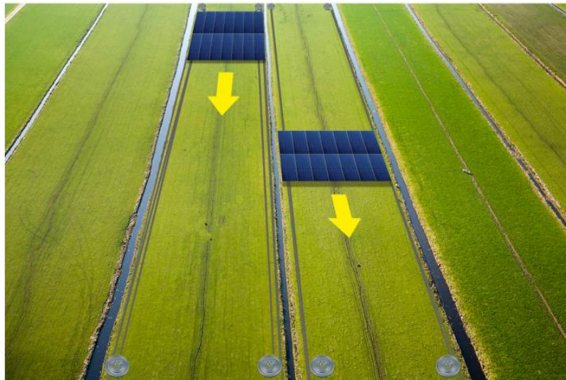
Figure 3: Schematic overview of the agrivoltaic system on a rails. On the bottom of the image are rotary electric engines that move the PV-panels on the rails. Parallel to the small (vertical) trenches are the rails anchored on the ground. The PV-panels are mounted on the rails at a height of 4m (not yet clearly visible). This diminishes the interference with the daily activities of the farmers. (own work)
