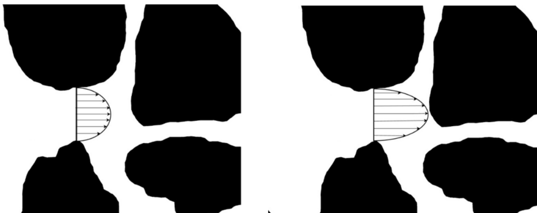
Figure 3.8 Flow velocity distribution between grains, with on the left-hand side a lower flow velocity and on the right a higher flow velocity
