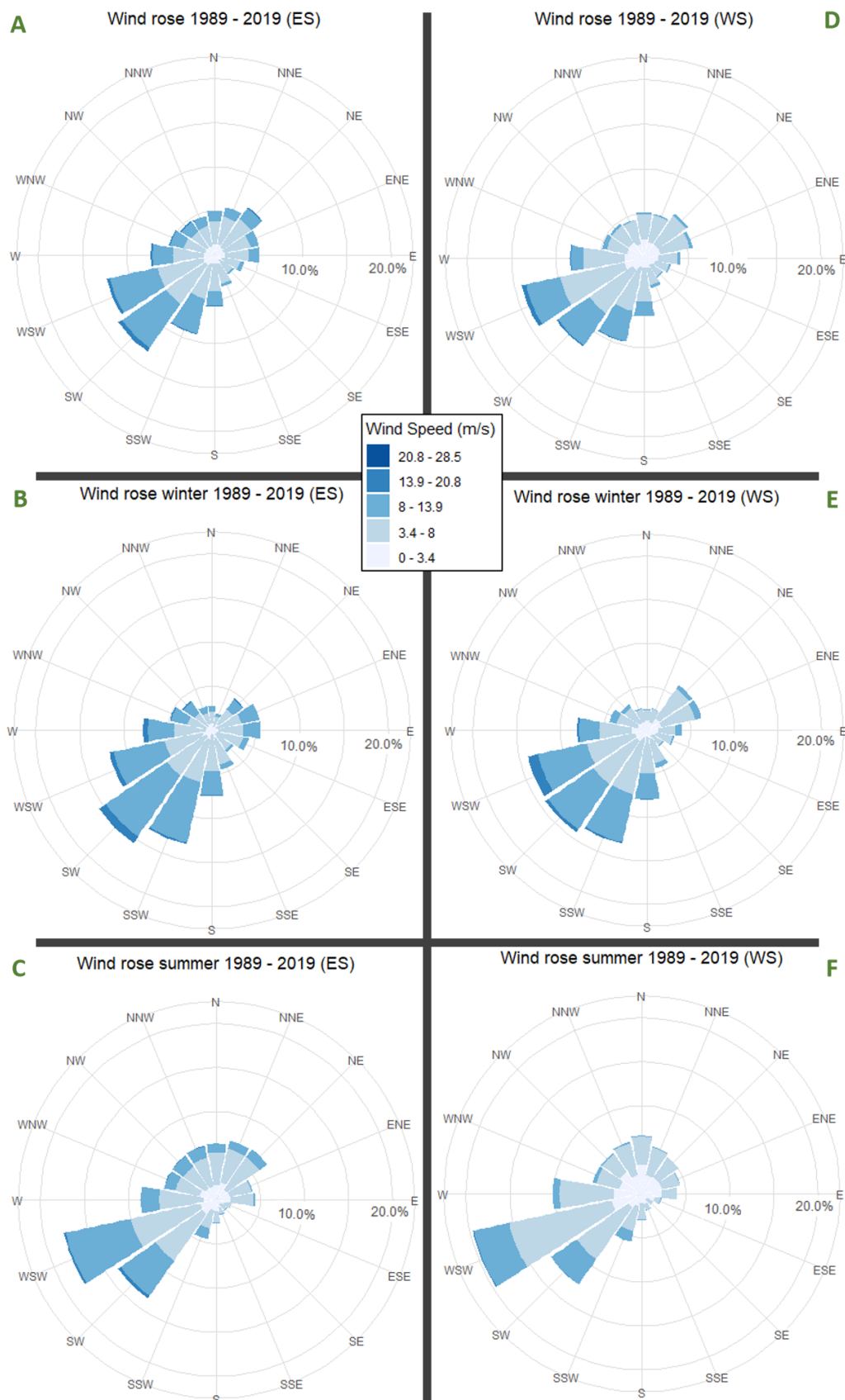
Figure A3 – Wind roses for the Eastern- and Western Scheldt, providing with the speed and frequency from 30 year of data. The Western Scheldt data is derived from station 310 (Vlissingen) and from 312 (Oosterschelde) for the Eastern Scheldt. The total average data is provided (A, D), and the winter (B, E) and summer data (C, F).
