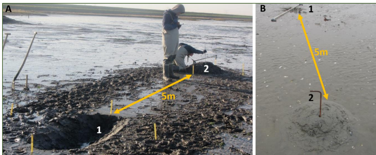
Figure A2 - Pilot studies for the disturbance and recovery experiment; (A) shows the first pilot study. A hole (1) and a pile (2) of sediment at Rattekaai (25m). The relative height of the pile is measured by means of a SEB. (B) shows the second pilot study with a smaller hole (1) and pile (2) of sediment. The relative height is measured by the height of a stick
