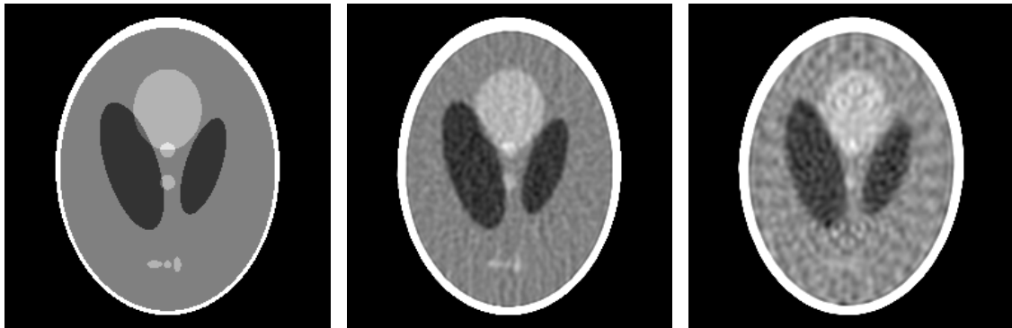
(a) Modified Shepp-Logan phantom. (b) Smoothed FBP (290 projections). (c) Smoothed FBP (58 projections).
