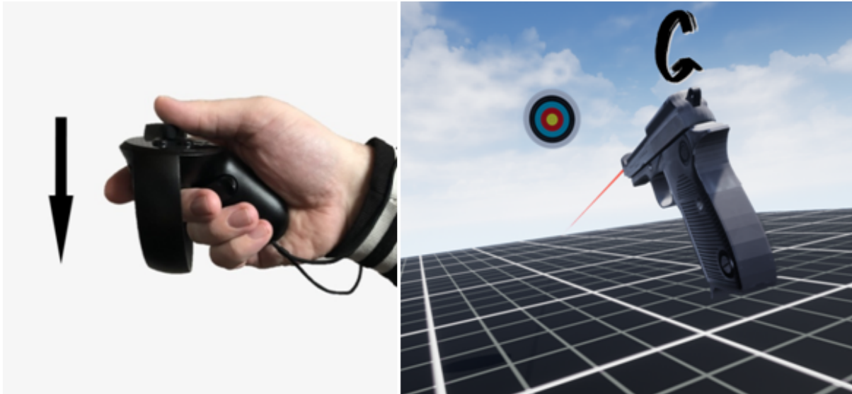
Figure 6: Aiming with Gun. Moving the Oculus Touch will move and rotate the gun.
