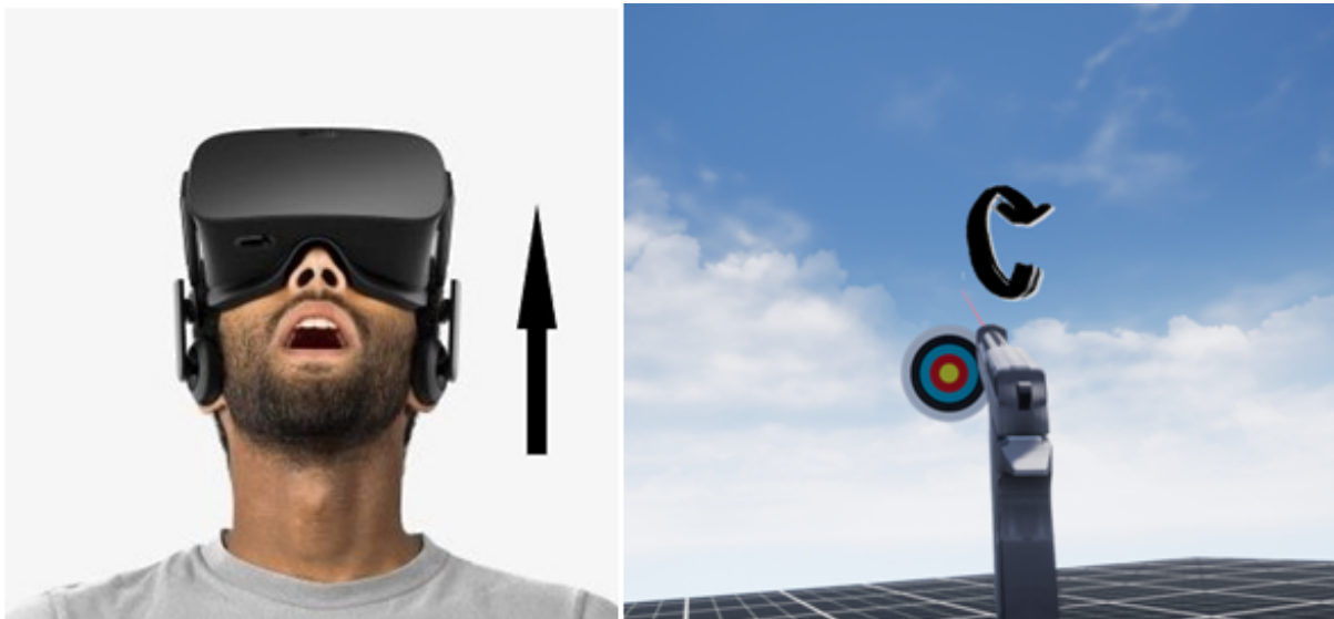
Figure 5: Aiming with Head. the gun and camera are controller by the head movement.
