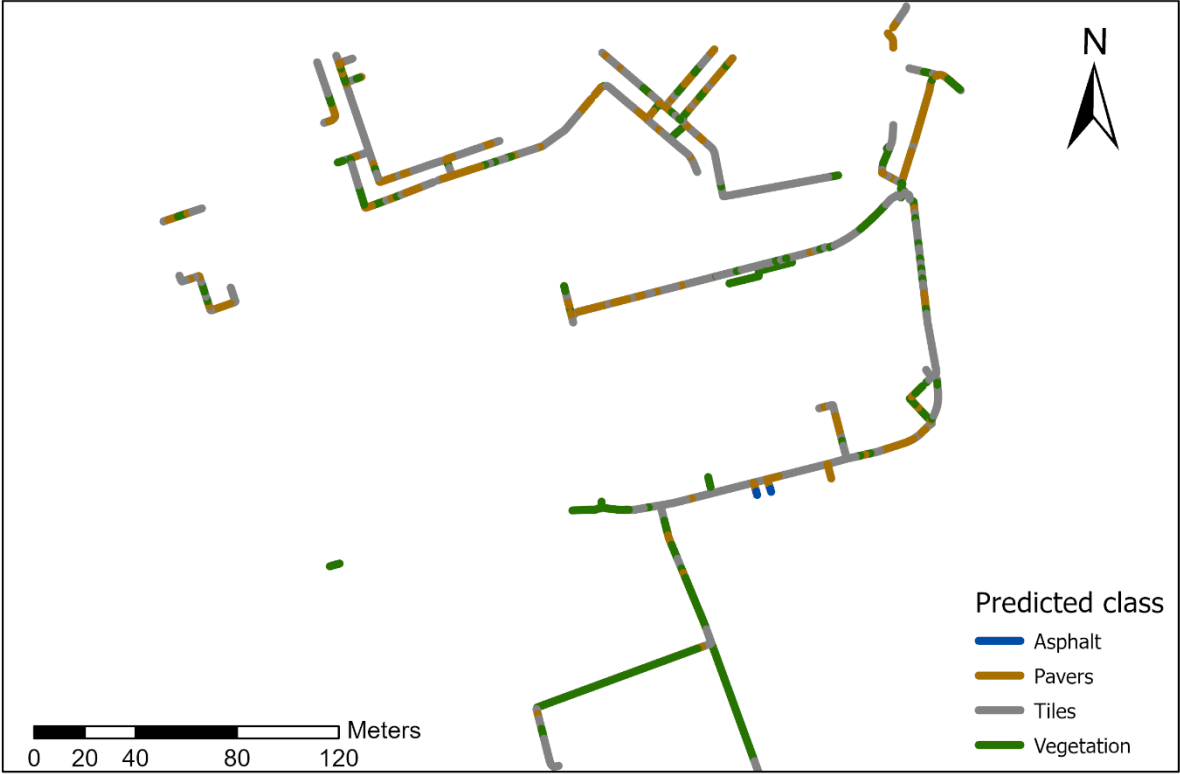
Figure D.1. Visualization of the predicted urban land cover of each cable segment by the non-augmented model.
