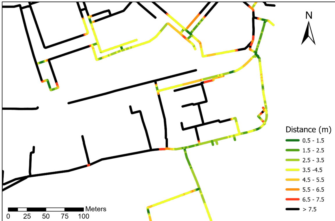
Figure C.1. The nearest distance between cable network segments and the image capture locations in a range of 7.5 meters.
