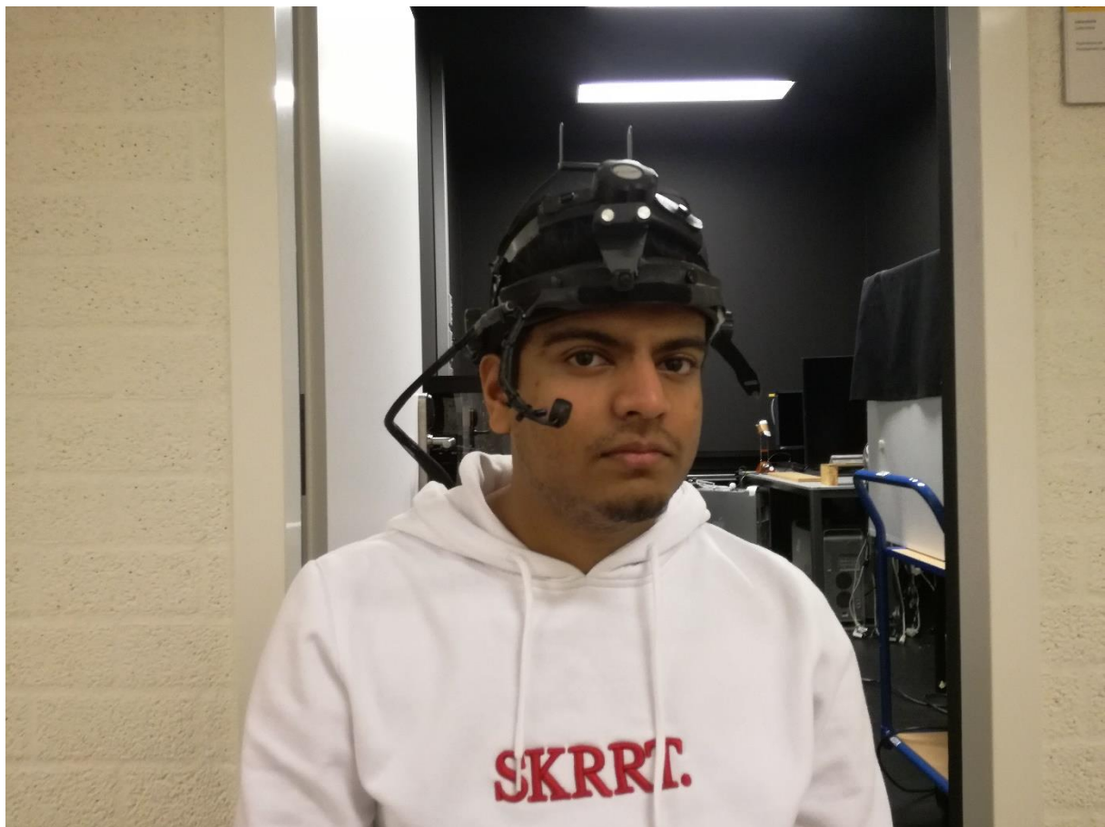
Figure 2 Participant wearing the positive science wearable eye tracker on a custom mount fit for adults
