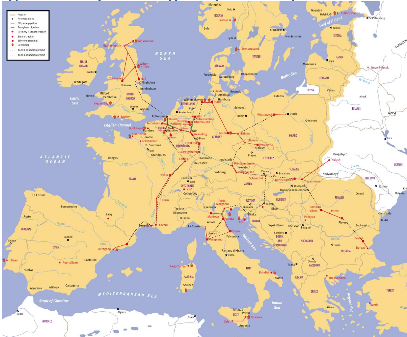
Ethylene and Propylene pipelines in Europe today and in the future (Association of Petrochemical Producers in Europe, 2009)
