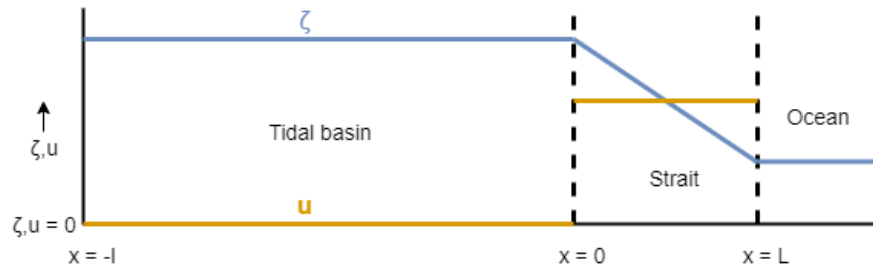
Figure 6: Side view of a Helmholtz basin, following the same basin geometry as the basin in Figure 5. In the first order, the water level \zeta (blue) is constant in the basin and linearly decreasing in the strait, while the velocity u (orange) is zero in the basin and constant and positive (towards the ocean) in the strait. This depicts the positive phase of the Helmholtz mode. In the negative phase, the water level increases linearly in the strait and the velocity is negative.
