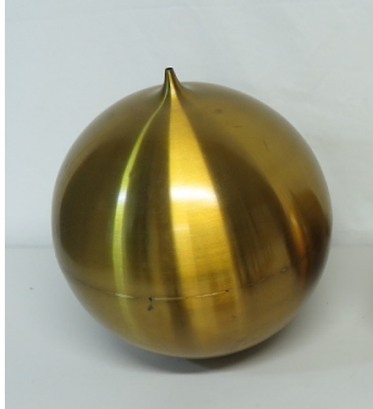
Figure 3: Helmholtz resonator, consisting of a nearly spherical container and connected through a small neck with hole to its surroundings. From The National Museum of American History (2020).
