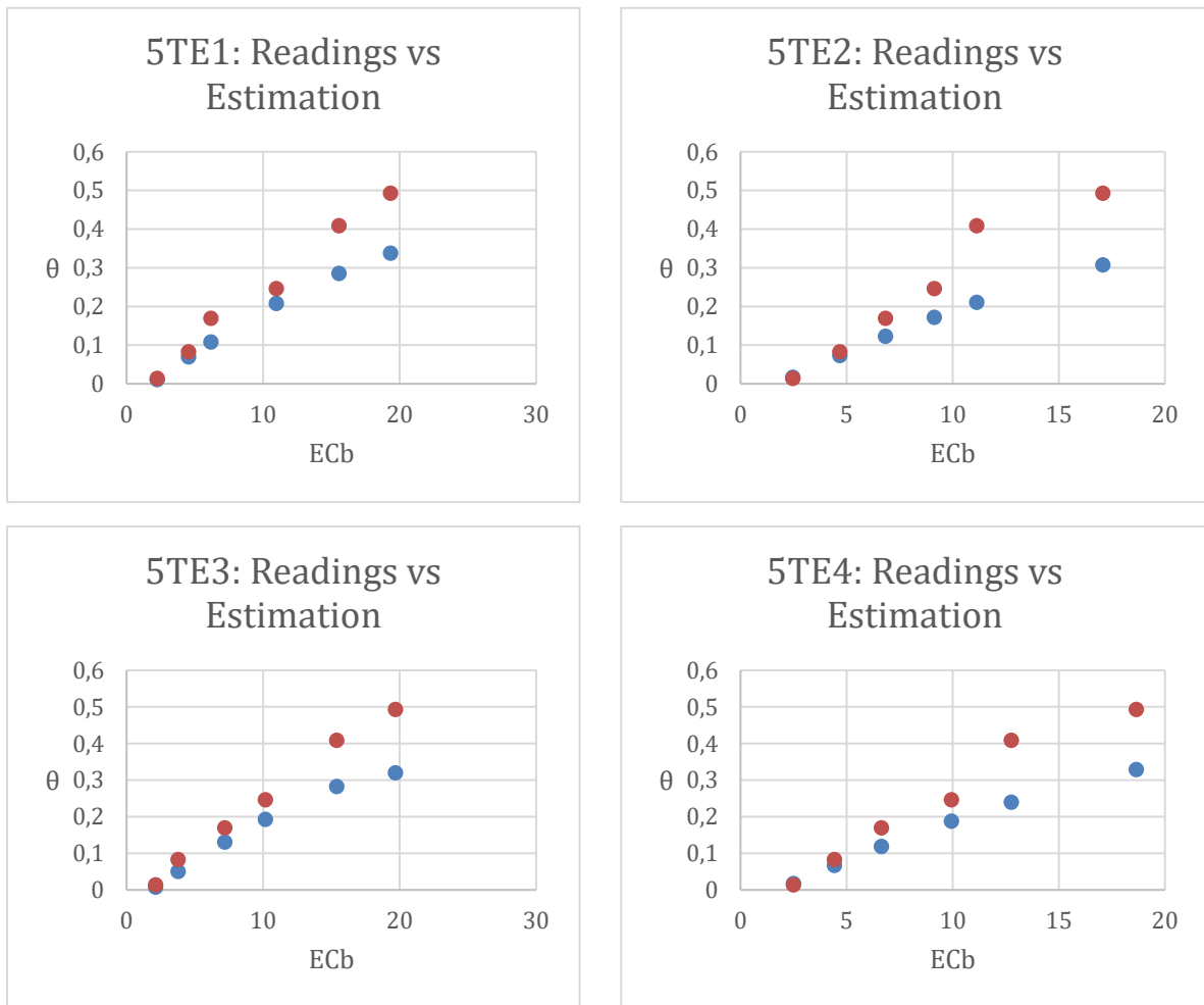
Figure D-1: 5TEs calibration curve vs raw data curve
