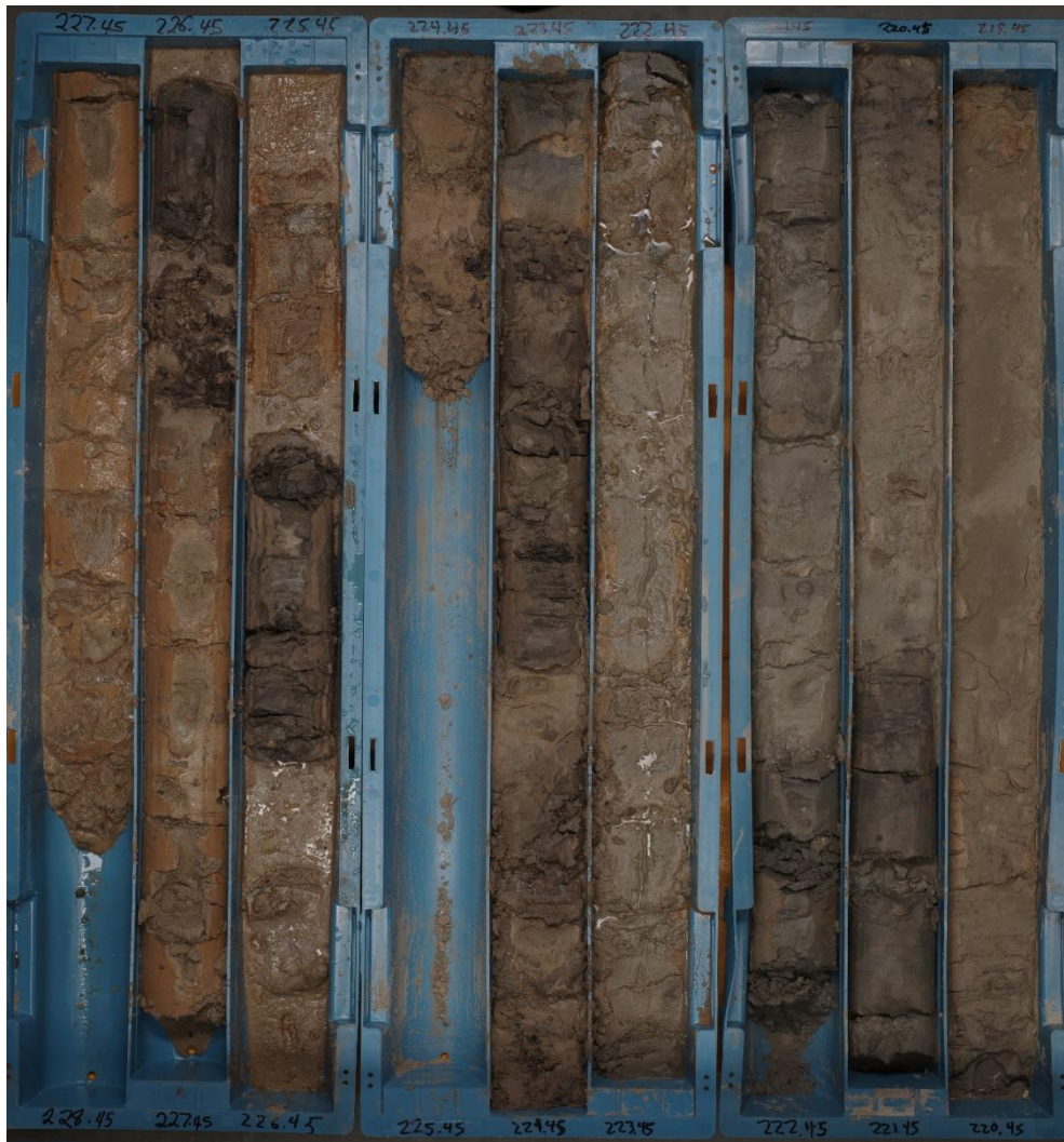
Fig. 2.5 Abrupt lithology changes in the interval 228 – 220 m, in fluvial environment. Some changes are more abrupt, leaving a clear contact, while the others are more gradual.
