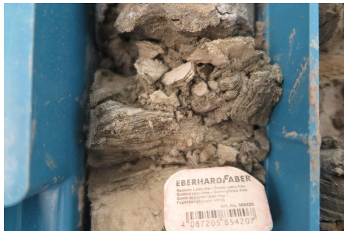
Fig. 1.14 222.23 m. Very thin alternations of clay and sand, could be tidal formation.
