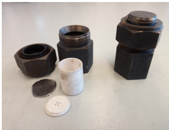
Figure 12: Photograph of reactor components used for carrying out melt infiltrations with LiNH 2 , showing a white ceramic container, grey graphite foil and stainless steel reactors.
