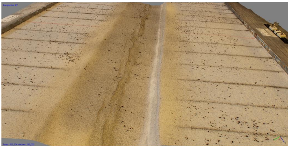
Figure 2.1.39. 3D perspective view of the extension graben.
