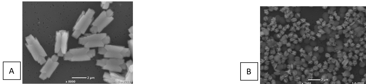
Figure 42: Tabletop SEM results with additional NaCl as BE baryte mixtures with a [Ba^{2+}]:[SO_4^{2-}] ratio of 0.001 (A) and 1000 (B). Both solutions were grown at \Delta\mu = 4 .
