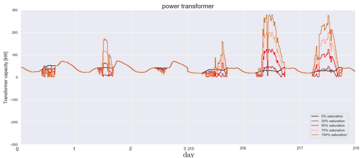
Figure 17: Network interaction and transformer capacity of the reference PV scenario with different saturation rates of 3 winter days (1,2,3 January) and 3 summer days (3,4,5, Augustus).
