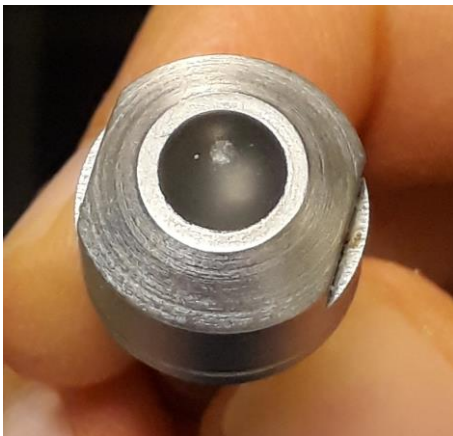
Figure A 18. Image of the ball holder with a PDMS probe after a tribological measurement on a rubber substrate at 0 N. There is a wear spot present on the probe. Before the measurement, the probe was brought in touch with the substrate with 0.08 N normal load, and then the UMT TriboLab retracted the probe until it measured a load of 0 N.
