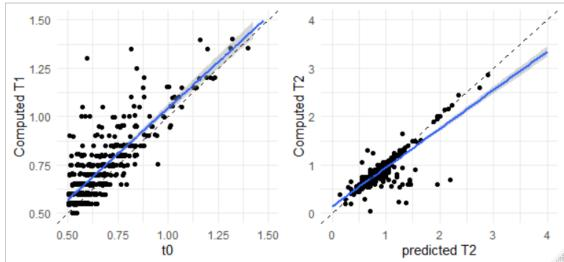
**Figure 8**. The TPVCM predicts initial (T1) and final (T2) reaction times. A. Correlation between the T1 computed from the data and delay period  $t_0$  from the model. B. Correlation between T2 computed from the data and T2 predicted by the model. The blue lines indicate regression lines; The dashed lines indicate identity lines.
