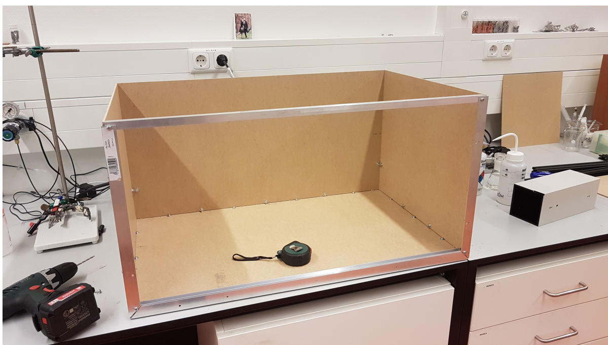
Figure A.3: Image of the blackbox of the photo electrochemical set up during construction
