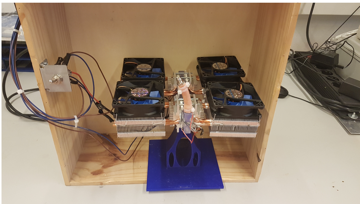
Figure A.1: Image of the cooling system constructed with peltier cells
