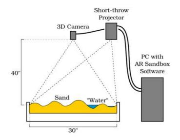
*Figure 2-* The arrangement of projector and sensor to project colours over sand. Retrieved from UC Davis' manual for construction of AR sandbox, <u>https://arsandbox.ucdavis.edu/instructions/hardware-</u>2/
