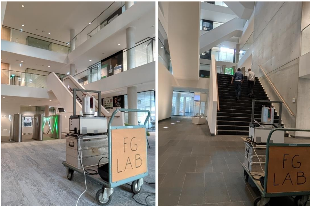
Figure 45: TLS set up in Vening Meineszbuilding. Left: Scan position 1. Right: Scan position 2.
