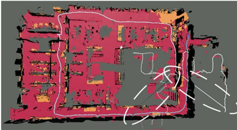
Figure 52: indoor environment of the building of Architecture of Delft University of Technology. This environment is regarded to be visual feature sparse, due to the large open space in the middle of the scanned environment. The right bottom corner shows two cases of tracking loss, displayed by the completely straight tracks.
