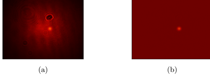
Figure 23: The left image (a) shows the full interference pattern of a measurement. The right image (b) shows the same image but with the reference beam, as measured at the start of the run, removed after rescaling.
