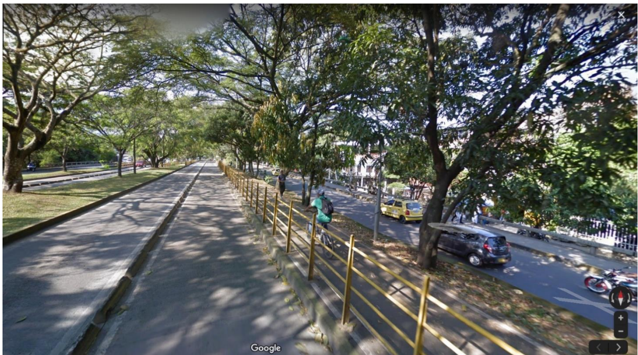
Figure 17 Separated cycling lane in Cali, Colombia. The middle two lanes are bus lanes. Calle 5, Cali, Colombia. From: Google Maps Street View.
