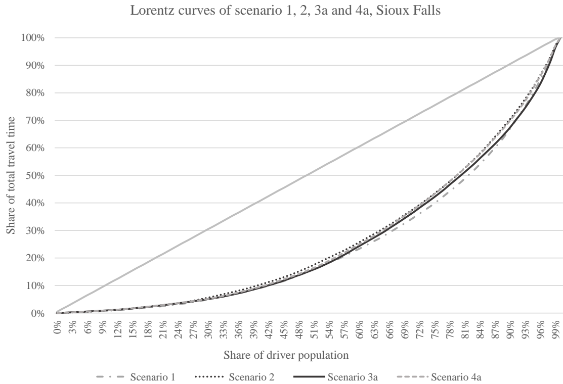
Figure 4.25: Lorentz curves of scenario 1, 2, 3a and 4a, Sioux Falls. The linear line from (0,0) to (100,100) is the line of equal distribution
