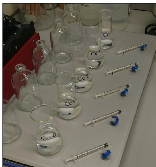
Figure 4. Set-up of the bulk dissolution experiment. The septum bottles used to transfer the sodium chloride solution to the experiment are shown on the far left. In the middle row are the sample beakers containing the stirring bar, sample powder and sodium chloride solution. The syringes and filter used for sample extraction are on the right.
