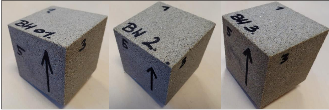
Figure 3. Cubic samples BW-01, BW-02 and BW-03, used for the experimental procedure in the multianvil apparatus at the Christian-Albrechts University. All cubes have a diameter of ~43 mm, arrows indicate the bedding direction.
