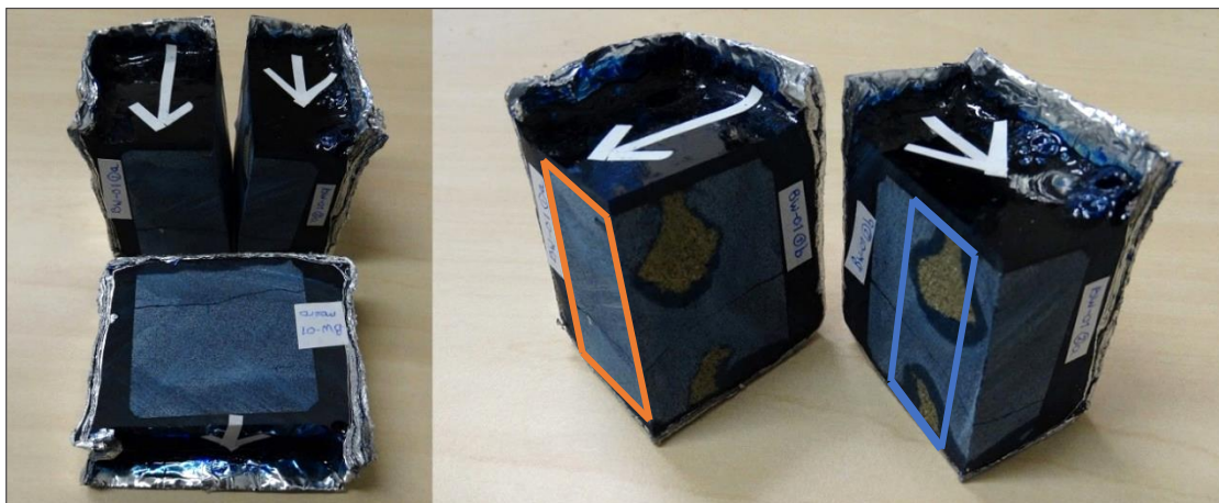
Figure 9. Sample BW-01, cut after a first impregnation attempt. The white arrows correspond to the white arrows indicated in Figure 7 . Chosen surfaces for further thin section analysis are indicated: BW-01-1-a (red) and BW-01-2-b (blue), oriented perpendicular to each other and to the experimental Z-direction.
