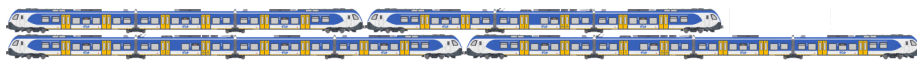
Figure 2.2: The upper train consists of two units of type ‘Flirt3’ while the lower train consists of two units of type ‘Flirt4’. Both trains are of the same type, namely ‘ Flirt ’ but are of a different sub-type.
