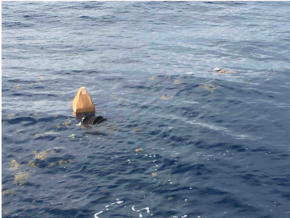
Figure 3: During the span of 17 days in the summer of 2019, 20 undrogued Stokes and 18 drogued SVP drifters are released in the North Atlantic sea to track Sargassum. On the left we see a drogued SVP drifter and on the right we see an undrogued Stokes drifter. Photo taken by Erik Zettler [6].
