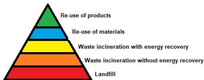
Figure 10: The ladder from Lansink, named after Ad Lansink, a Dutch politician who filed a motion in 1979 to work according to this hierarchy. This shows the hierarchy of treatment options for solid waste, the least preferred option is landfilling and the best option is to reuse products without the need for recycling.
