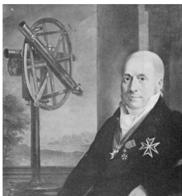
Figure 1: Painting of Krayenhoff [Haasbroek 1972, p. 7, 13] with his repeating circle on the left.
