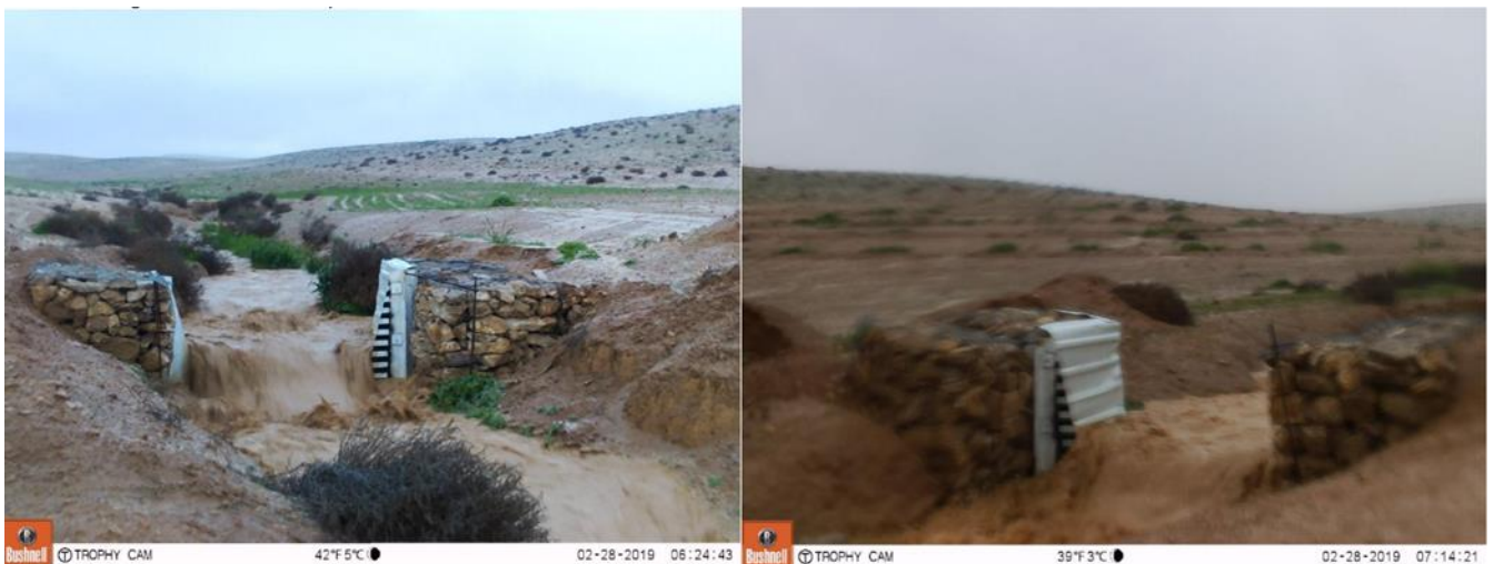
Figure 27: Peak discharge event in the untreated (left) and treated (right) watersheds at 28-02-2019.
