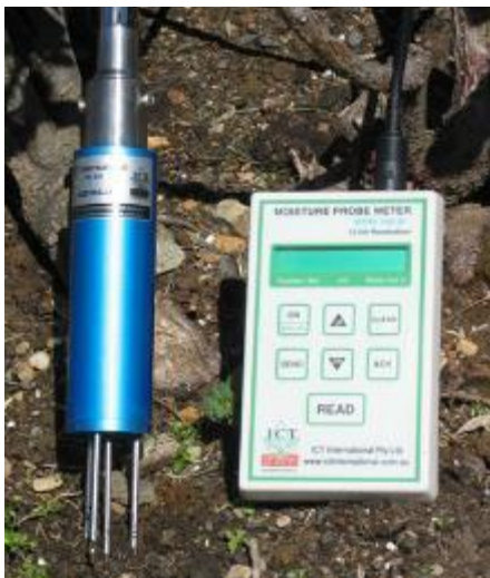
Figure 11: The handheld MP306 ICT TDR used to measure soil moisture content in the soil.
