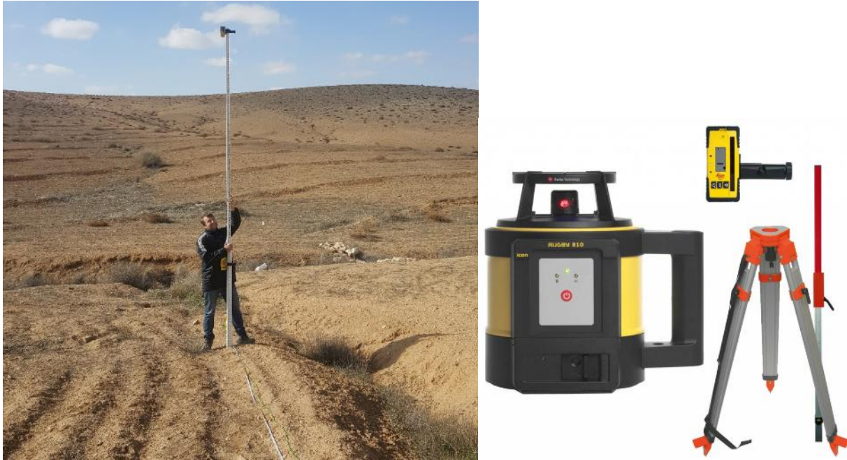
Figure 9: The measurement bar (left) and the Leica Rugby 810 laser level altitude meter and receiver (right).
