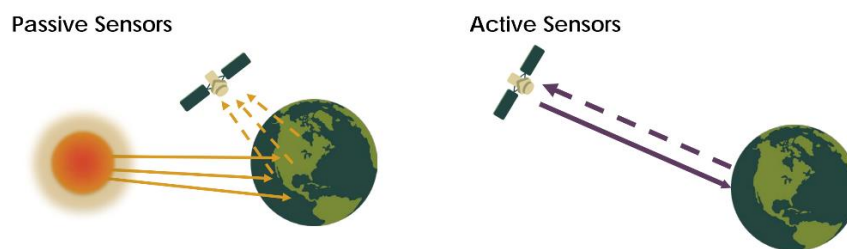
Figure 2.5 Diagram of a passive sensor versus an active sensor (Applied Remote Sensing Training, n.d.).
