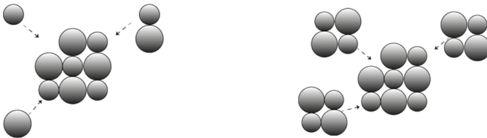
Figure 2.4: left: Single ion or building block addition, critical nuclei growth according to classical nucleation theory. Right: Coalescence of multiple pre-critical nuclei to form a supercritical nucleus.
